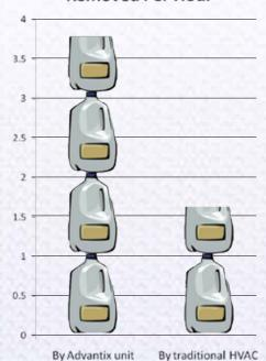
CrossFit ATP accommodates about 70 members an hour during peak workout sessions, which produces approximately 63 gallons of moisture. An Advantix Systems DT-800 unit removes up to 88.8 gallons per day; compared to just 38.4 gallons removed by a conventional system.
